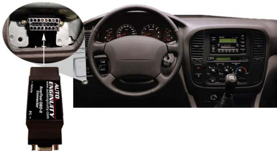
3. Connect the “Vehicle” end of the AutoEnginuity ProLine VCI connector to the vehicle’s DLC.
